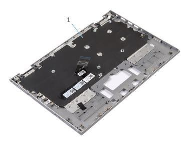
1 palmrest and keyboard assembly 2 screwTurn the palmrest and keyboard assembly over and keep it aside.
